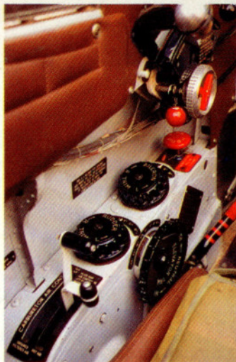
The three trim wheels (left) are clustered together, and the rudder pedals (below) are adjustable fore and aft for tall and short pilots.
