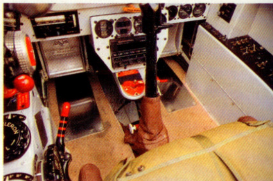
The three trim wheels (left) are clustered together, and the rudder pedals (below) are adjustable fore and aft for tall and short pilots.
